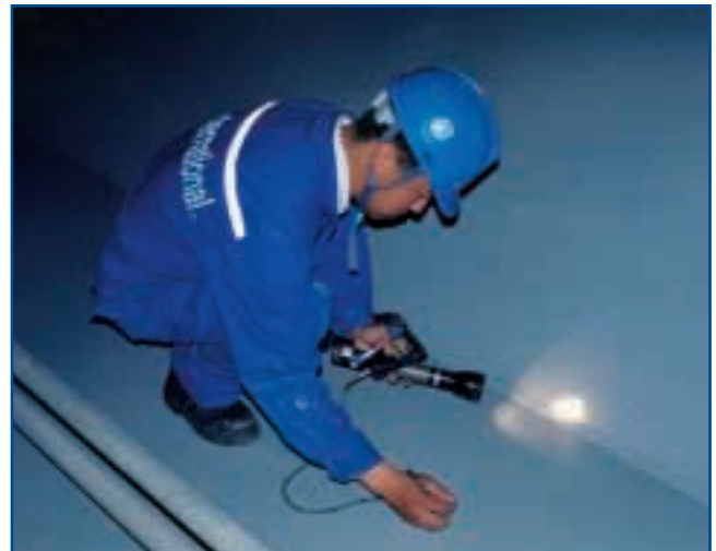
Dry film thickness measurement.
