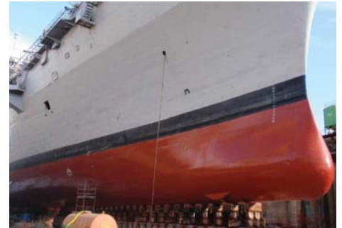
Principe de Asturias reported a speed increase of 3 knots after Intersleek®900 application
