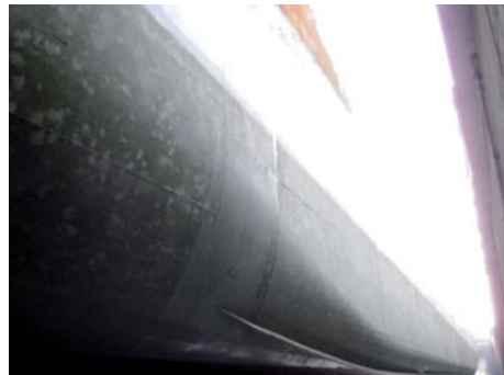
Intersleek 900 test patch on VLCC after 59 months
