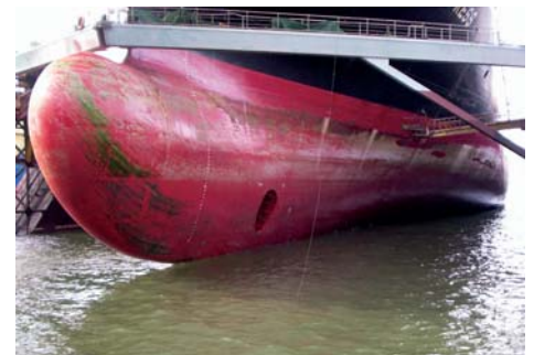
Container vessel after 60 months before washing
