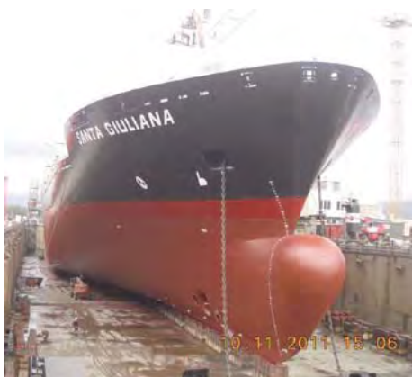
'Santa Giuliana', coated with Intersmooth ® 7460HS SPC, Besiktas Shipyard, Turkey in November 2011
